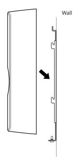
**3** Connect BioEntry P2 to the bracket by rotating the product fixing screw.
